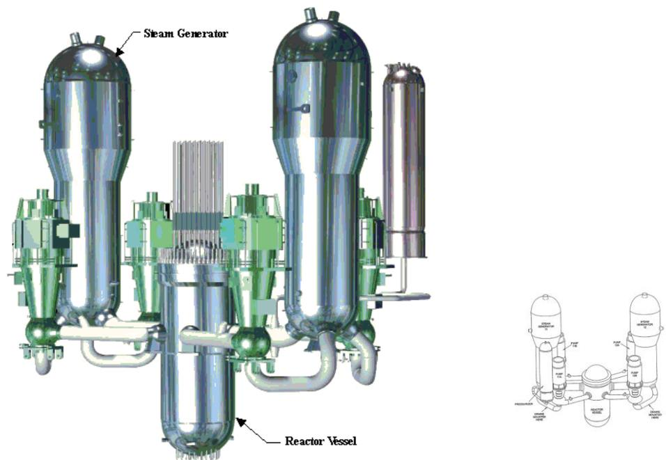
**FIGURE 2B TYPICAL TWO-LOOP COMBUSTION ENGINEERING UNIT**
