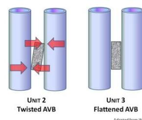
23 This distortion occurs when the length of bar is wrapped back on itself to form the ‘V’ or hairclip shape, with the bar warping particularly towards the nose section. For Unit 2 the AV bars were subject to a pressing flat force of ~3 tons, but this did not completely flatten the bar so for Unit 3 the pressing force was increased to ~10 tons.
