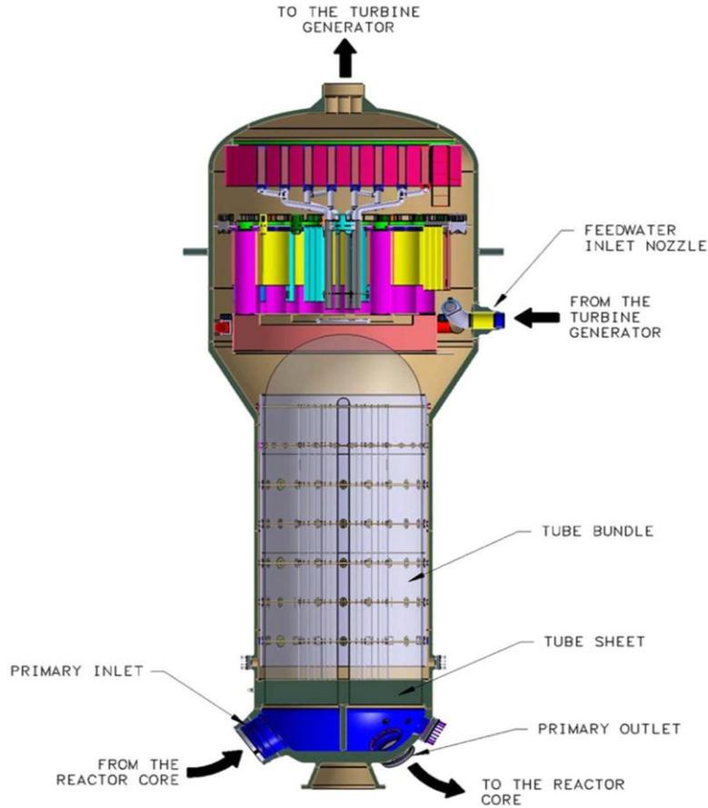
**FIGURE 1A MHI REPLACEMENT STEAM GENERATOR**
