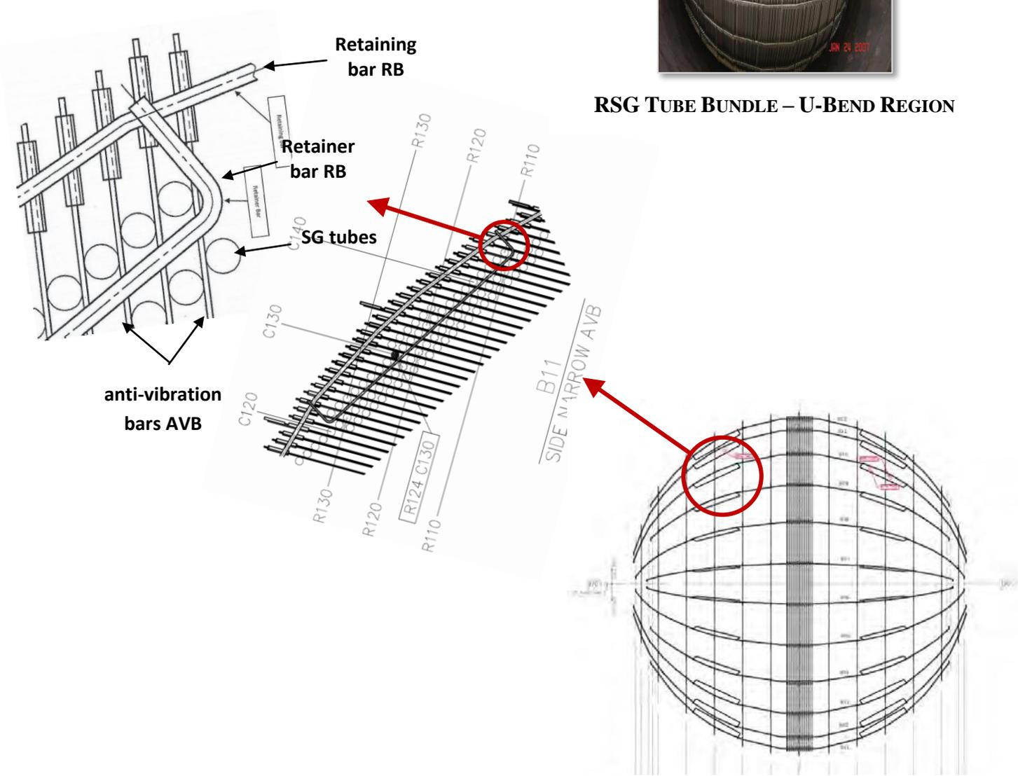
**FIGURE 5 ANTI-VIBRATION AND RESTRAINT BAR ASSEMBLY**
