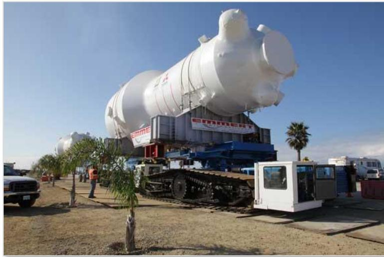
**FIGURE 2A MHI REPLACEMENT STEAM GENERATOR IN TRANSIT**
